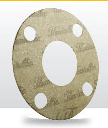
Thermiculite® 815 is a high temperature, chemically resistant sheet sealing material comprising exfoliated vermiculite reinforced with a tanged stainless steel core.
